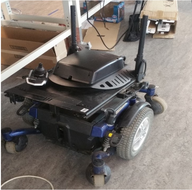
Figure 1. Wheelchair with only its seat stripped off
