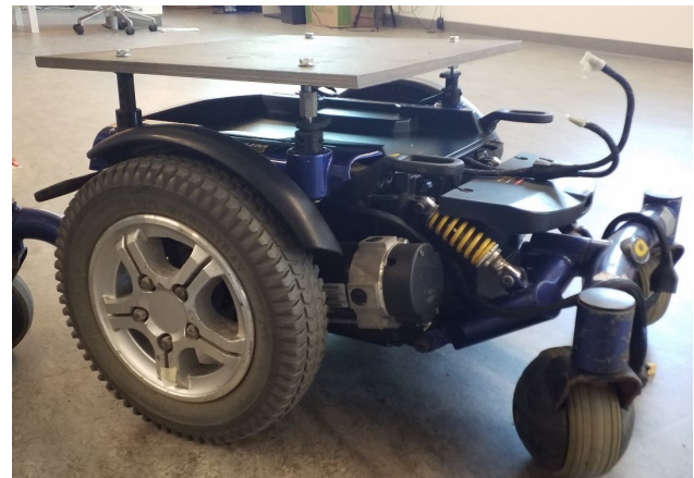
Figure 4. Hard-steel plate mounted onto power base
